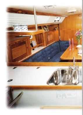
The galley and main cabin have received special attention to design and detail. The galley is a functional 'U' shape, with composite counter tops, sinks are near centerline for proper drainage underway. A large refrigerated ice box is aft and a dry food locker is forward. A gimbaled, stainless steel LPG stove with oven is standard equipment.
