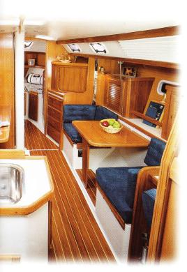
The main cabin can be arranged with a dinette or traditional table at your option. The two seats and game table to starboard can be made into a settee or berth with the cushions provided. The entertainment center cabinet can be fitted with a stereo and concealed TV. All interior teak has the warmth and durability only obtained with multiple coats of varnish.
